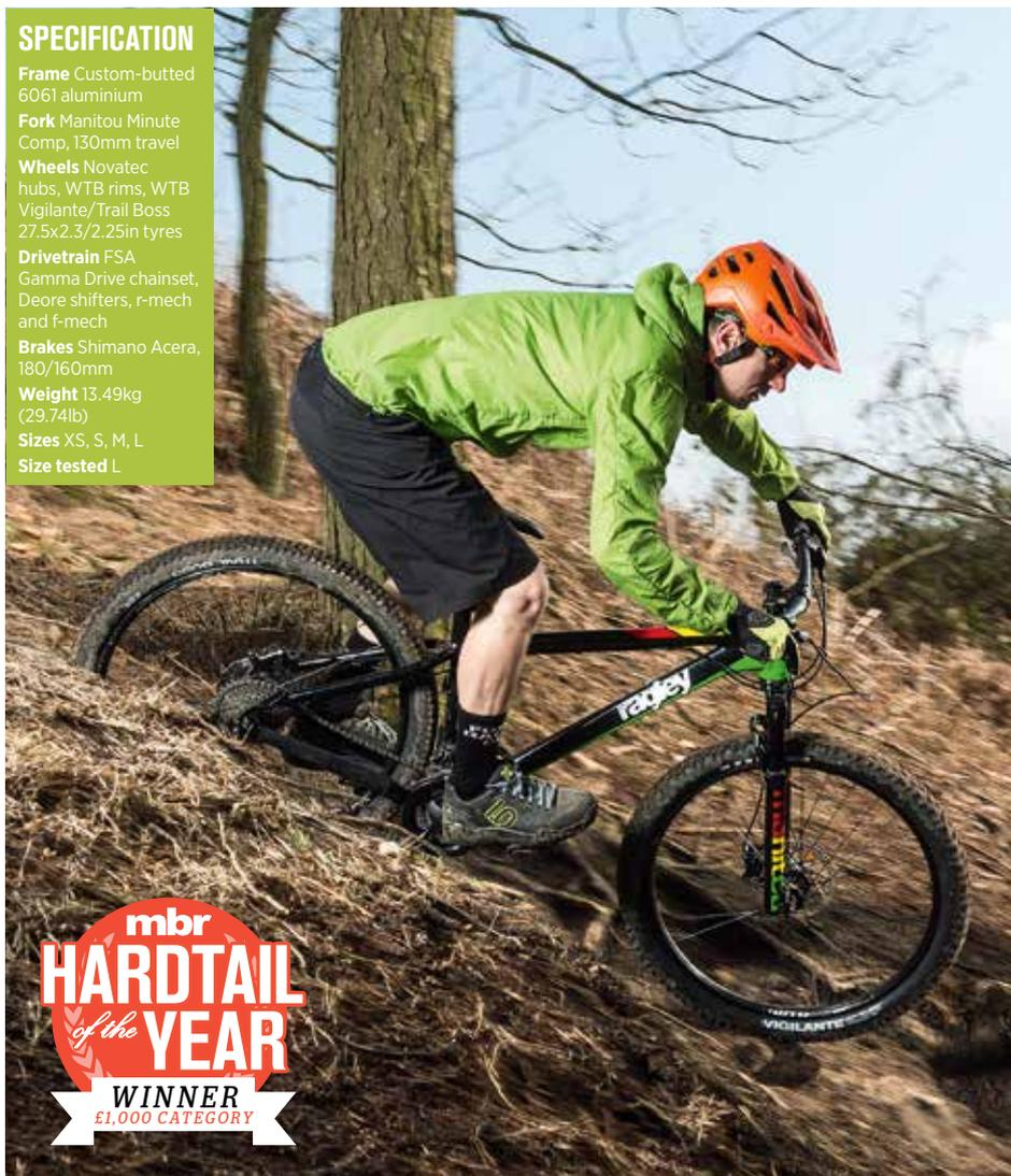
head angle means it never gets too twitchy on steep trails or under hard braking. The low bottom bracket allowed us to carve corners like no other bike on test, helped by the meaty front tyre and composed fork. Despite carrying a bit of extra weight, the seat angle was steep enough to let us tackle climbs without fuss, and the low-profile rear tyre helped cover ground efficiently.
