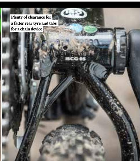
Plenty of clearance for a fatter rear tyre and tabs for a chain device
